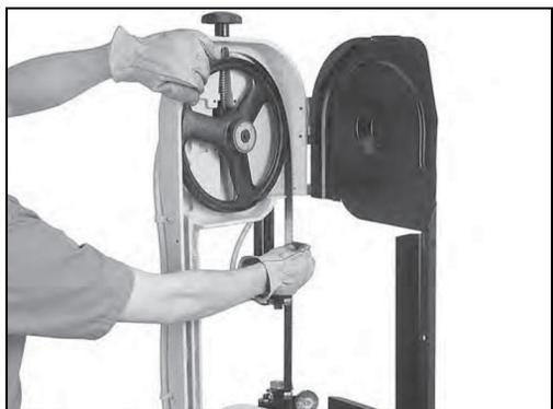
**NOTE:** It is possible to flip the blade inside out, in which case the blade will be installed in the wrong direction. Check to make sure the blade teeth are facing towards the workpiece, as shown. Some blades have a directional arrow as a guide.
